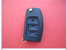
After removal of the old buttons pad, your remote should look like the one in the picture above, free of any old rubber pieces and dirt.
