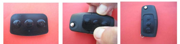
Place a new silicone pad over top part of your remote. Use rolling motion when positioning pad in grooves and press firmly till pad "engages" with hard shell all around edges and in the middle. If a new pad does not sit properly, remove it, clean grooves again and re-fit it. DO NOT USE any lubricants or detergents for cleaning grooves as it will affect firm seating of a pad. **No re-programming is need it** and remote will work straight away.
